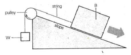
The block B rests on a slope. A string is attached to one end of the block and passes over a pulley at the top of the slope. A weight W is suspended from the end of the string.
