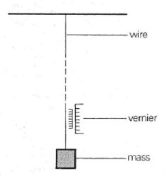
If the load is not too great, the wire will return to its original length when the load is removed. The wire is then said to be **elastic**.
