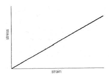
If the load applied is too great, the wire will not return to its original length when the load is removed. If this happens, the graph will not be a straight line. The maximum stress that can be applied for stress to be proportional to strain is known as the elastic limit. If the elastic limit is exceeded, the wire will not return to its original length. This is summarized by Hooke's Law, which states that:
