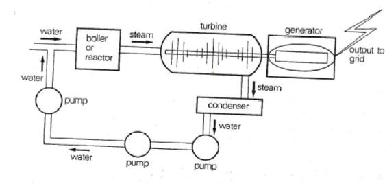
Steam is produced in either a boiler or a nuclear reactor. In the case of a boiler, this may be fuelled by either coal or oil.
