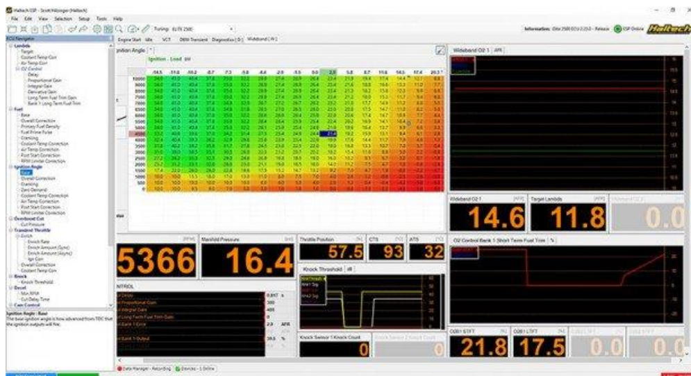
Fig.2.2.2.3. ECU's calibrating (reprogramming, remapping)
