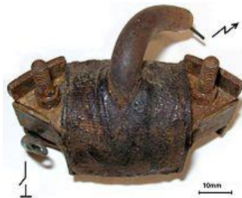
Fig.2.1.1. An early magneto-type ignition coil
