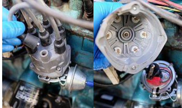
Fig.2.1.2.2. Distributor cap with wires and terminal. Rotor contacts inside distributor cap.
